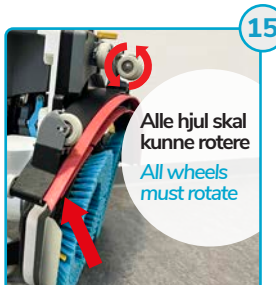
Tjek hjul for hår/snavs, og sugelæber for slid Check wheels for hair/ debris and squeegee for wear
