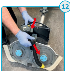
Tag sugeslangen af Remove the suction hose
