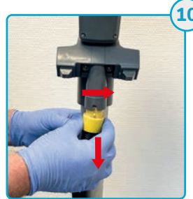
Skrue sugeslangen ud Unscrew the suction hose
